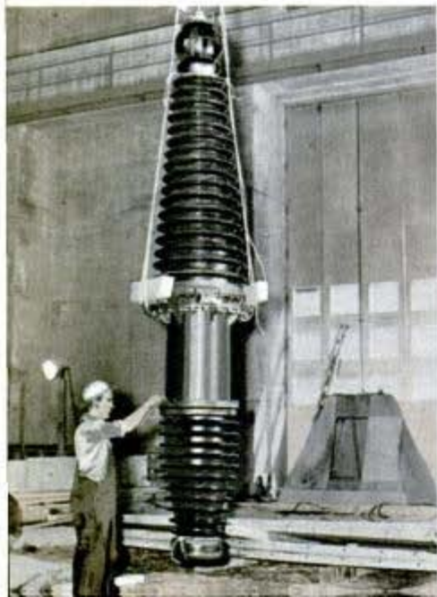
Another big item is the 16-foot-tall bushing, below, which is to be fitted into one of the transformers
